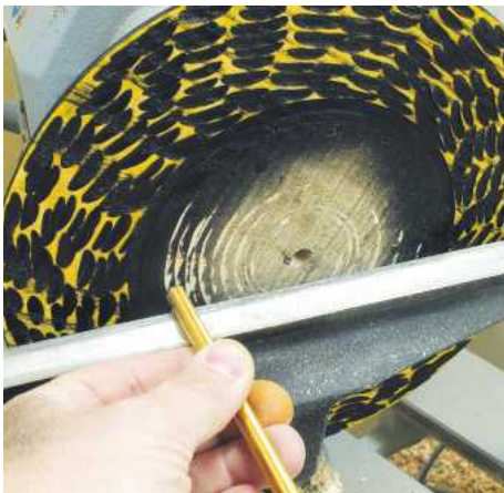
▲ Pic.22 When you have a decorated edge like on this bowl you will need to take extra care when making the first cuts. You can see how the tool has skated along the face
